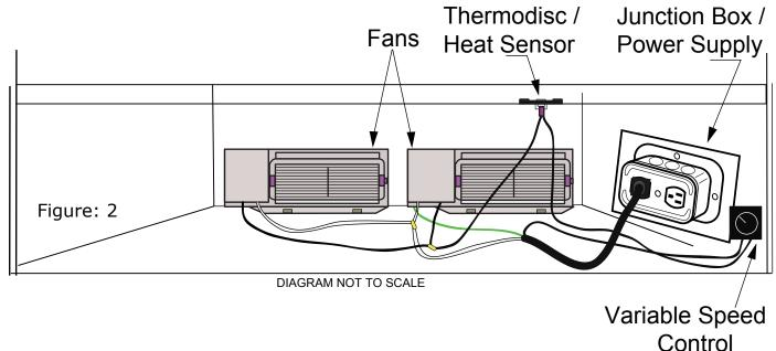
Finishing Steps: Plug power cord into junction box. (Figure: 2) If Appliance is connected to 120 Volt Power, turn power back on. Figure 3 illustrates the wiring diagram.
