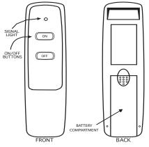
The transmitter operates on a 12V (A23) battery that is included. Install the 12V battery supplied with the unit into the battery compartment. It is recommended that ALKALINE batteries always be used for this product. Be sure the batteries are installed with the (+) and (-) ends facing the correct direction.
