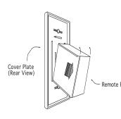
Position the receiver as shown in diagram to the left with lower tab on cover plate inserted into groove of receiver (Make sure LEARN hole on cover plate properly aligns with remote receiver). Pull receiver up and snap into top tab of cover plate.
