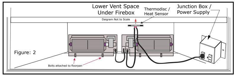
Finishing Steps: Plug power cord into junction box. (Figure: 2) If Appliance is connected to 120 Volt Power, turn it back on.
